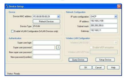
On the upper left corner, the MAC address of the KVM over IP module is displayed. To detect the MAC address, press the Refresh Devices button. The displayed MAC address should correspond to the printed address shown on the label on the base of the IP module.
